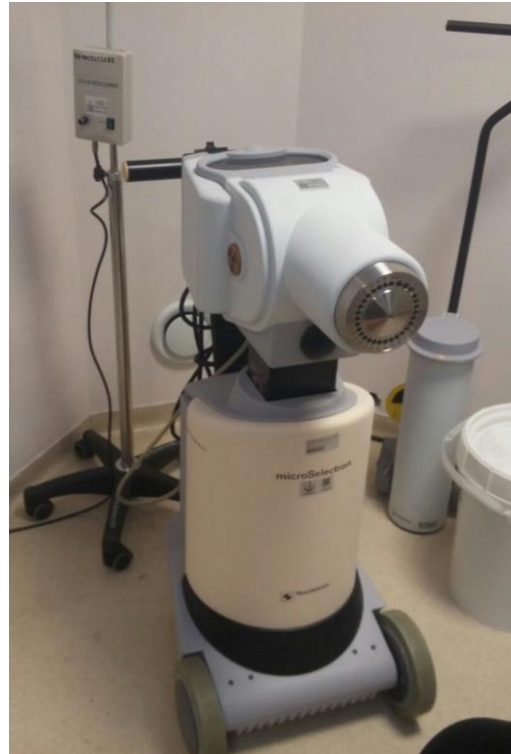
Şekil 4.1 microSelectron Digital® (ExBxG) ( 800x 980-1380 x 460 mm)
